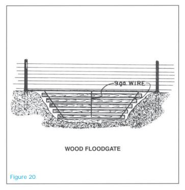
the bottom line wire to a depth equal to the water level or the lowest point of the ditch.
