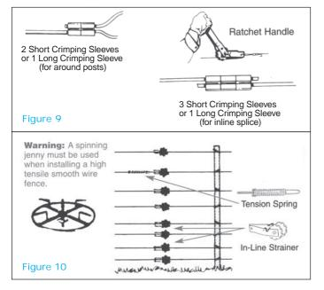
length of the fence to the next brace post. (Figure 10) Put a crimp sleeve on the wire (don't compress yet) then slide the wire through the wrap-around insulator. Wrap the insulated wire around the end post and compress the crimp sleeve. (Figure 9) Staple the wrap-around insulator to the end post.
